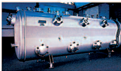
Fluid bed dryer for the production of raw material such as milk powder, lactose and citric acid.
