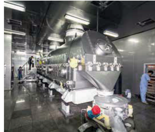
Vibration fluidized bed dryer used in the food industry
