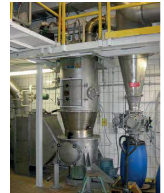
Dispersion dryer FL-T in the Allgaier Technical Centre
