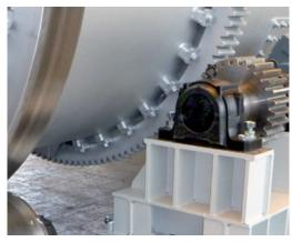
Gear rim drive of a rotating tube cooler
