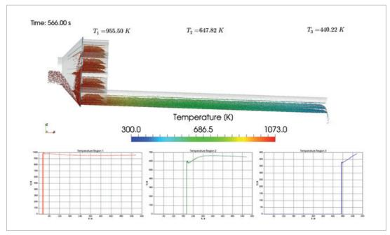
DEM computer simulation of cooling and movement of the solids
