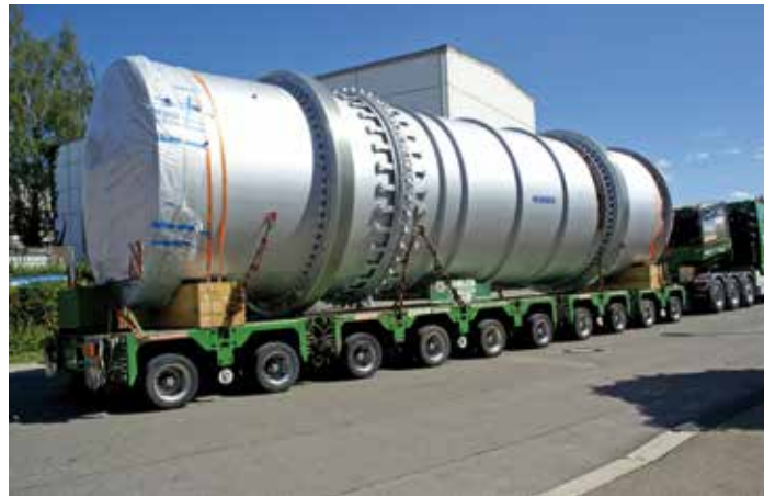
Drying-Cooling Drum for 100 t/h sand
