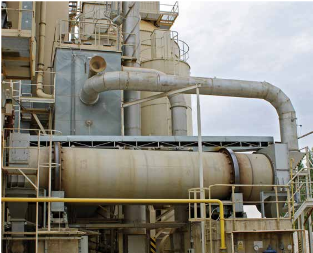
Drying-Cooling Drum for 100 t/h sand
