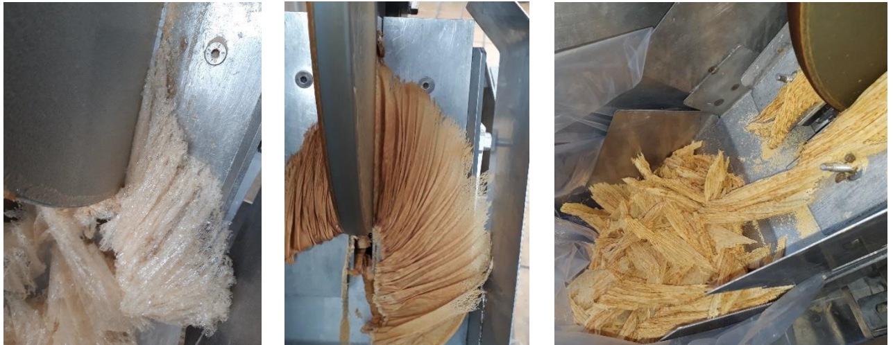
Figure 4: Examples of dry goods produced with the CDry (from left: beet pectin / brewer's yeast / protein suspension)
