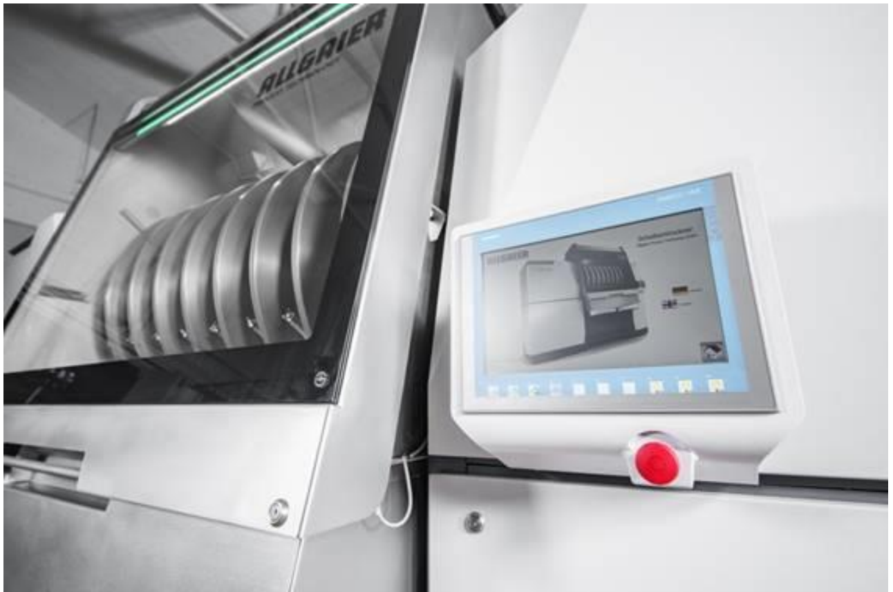
Figure 5: Intelligent system control via the intuitively operated touch panel for calling up and changing the current machine and process parameters.
