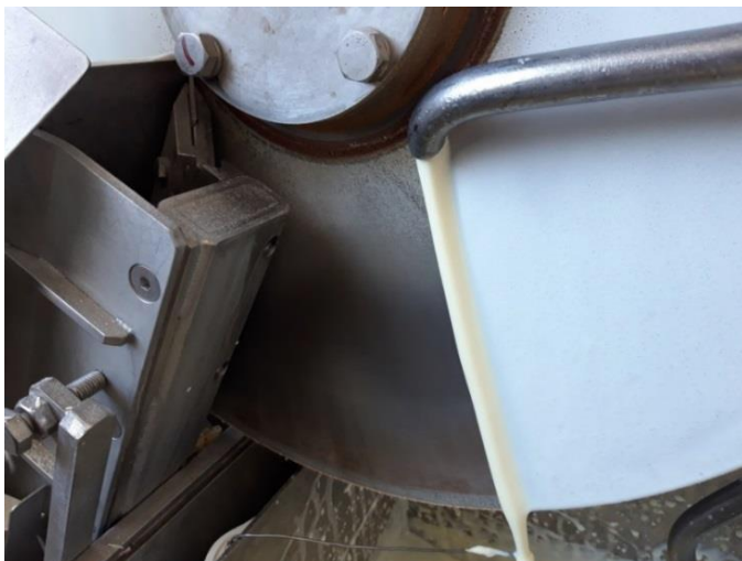
Fig. 1 and 2: Drying milk concentrate with the CDry 501 lab
