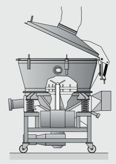
and maintenance. Both the air-director plate and the retaining sieve located in the upper part of the dryer can be removed very quickly by means of a hinged mechanism. These parts are held in position with quick-acting clamps.
