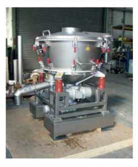
The round tank has a capacity of between 20 and 80 litres and the dryer can thus be used for the production of representative product quantities at low investment cost.
