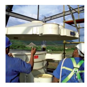
With the newly developed multi-dimensional electronic balancing system "MultiBalance", Allgaier have optimised the vibration characteristics of their tumbler screening machines even further. This new system makes it possible to eliminate the imbalance. Measurements have
