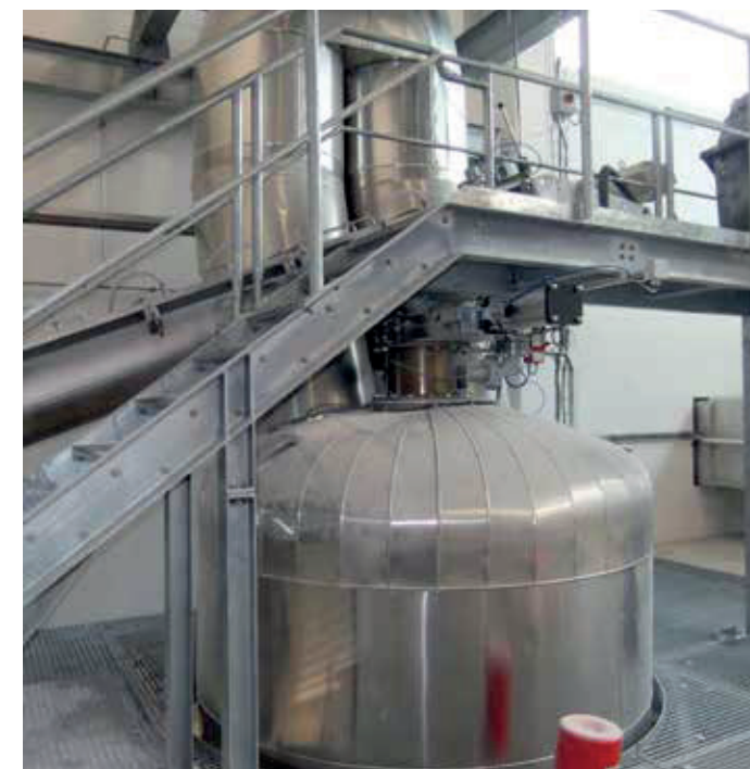
Dryer upper section with moist product infeed
