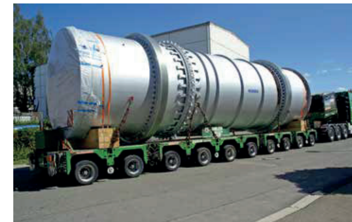
Drying-Cooling Drum for 100 t/h sand
