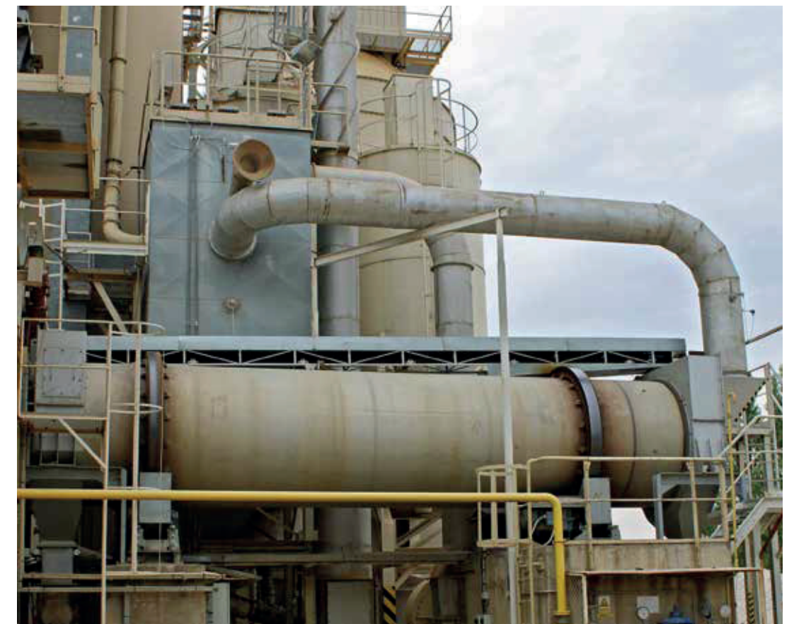
Drying-Cooling Drum for 100 t/h sand
