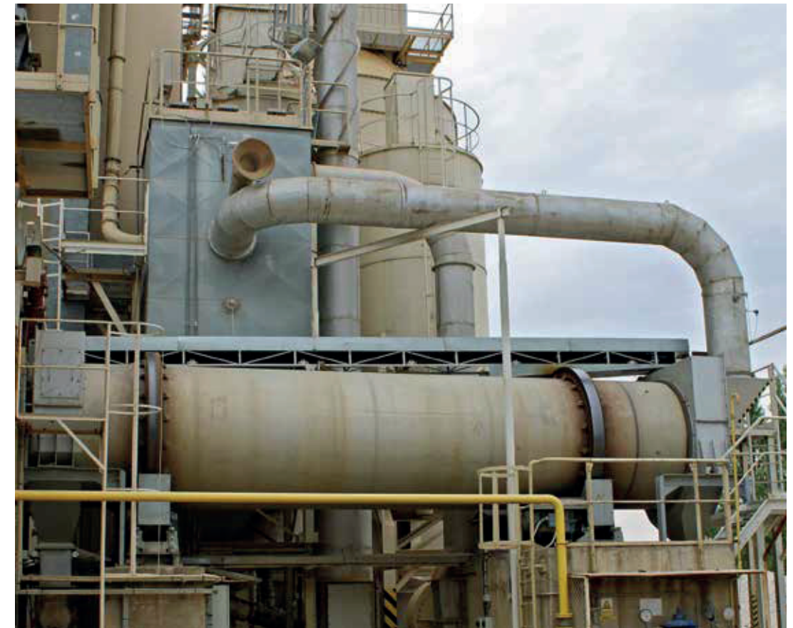
Drying-Cooling Drum for 100 t/h sand
