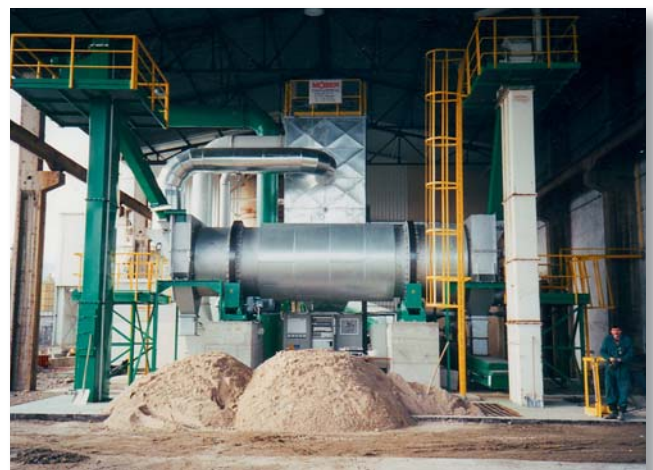
Figure 5: Drying/cooling rotary tube – MOZER® TK_plus system with moist sand introduced at both ends
