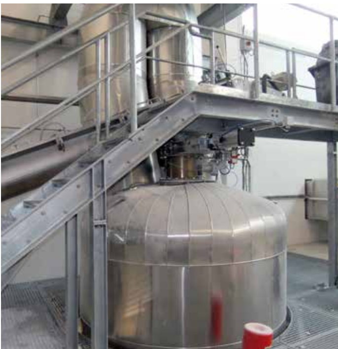
Dryer upper section with moist product infeed
