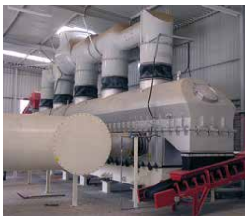
Vibration fluidized bed dryer for drying of mineral raw materials
