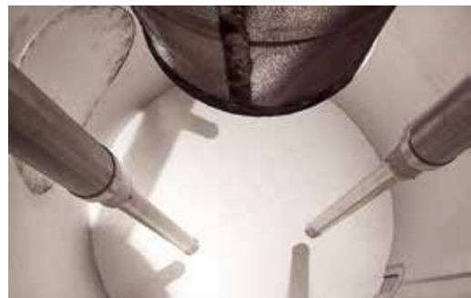
Suspension and paste dryer WS-IB-T for the creation of powders from liquids and pastes
