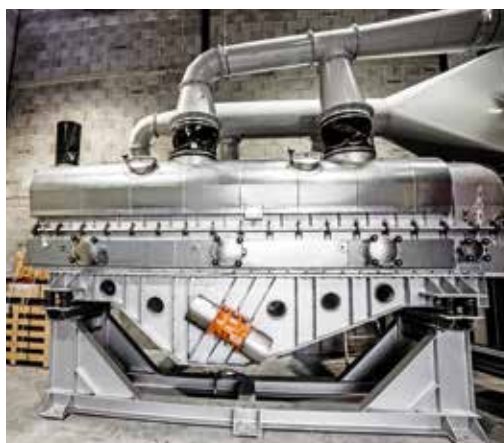
Fluidized bed dryer configured as free oscillating system for drying soot
