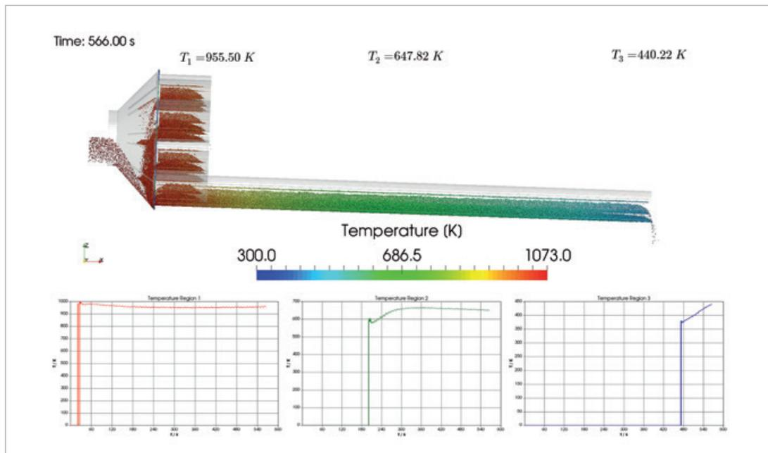
DEM computer simulation of cooling and movement of the solids
