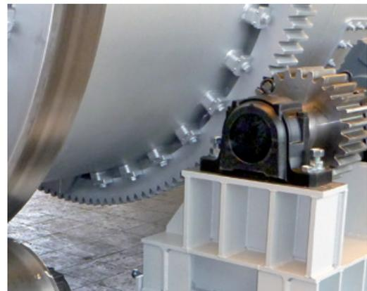
Gear rim drive of a rotating tube cooler
