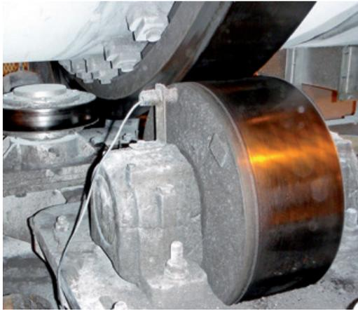
Roller station of a cooler for titanium dioxide in operation
