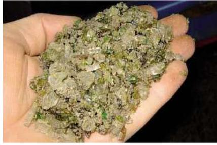
**Fig. 2: Recycled glass crushed to <math>< 10\text{ mm}</math> before cleaning and drying.**
