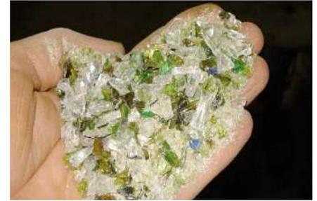
**Fig. 3: Recycled glass after cleaning and drying before the sorting process.**
