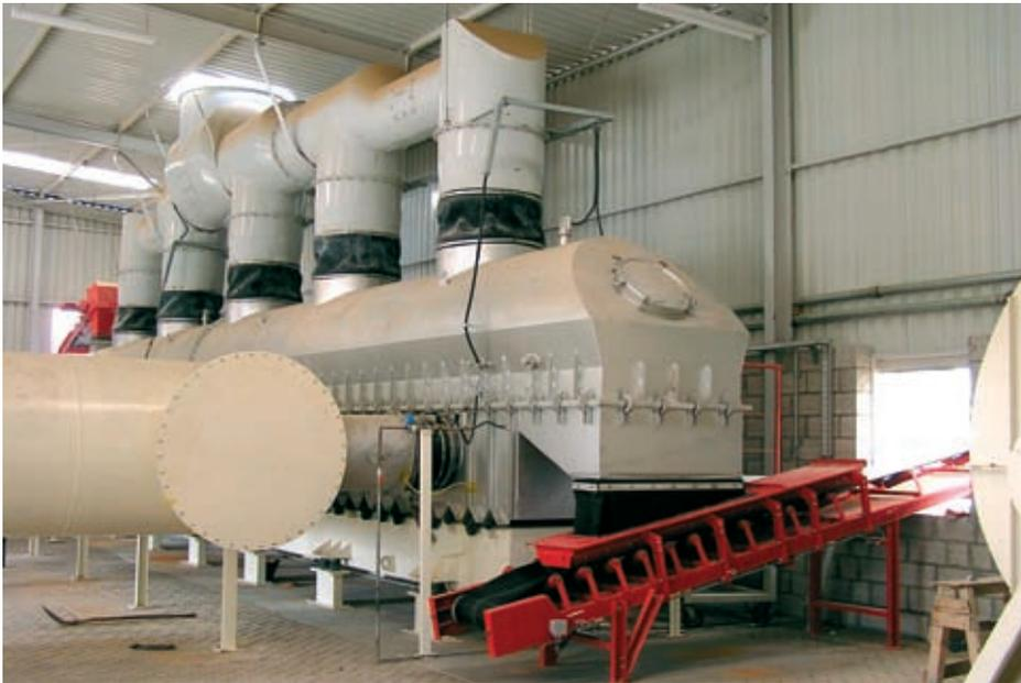
Fluidised-bed dryer for drying sand, limestone and marble
