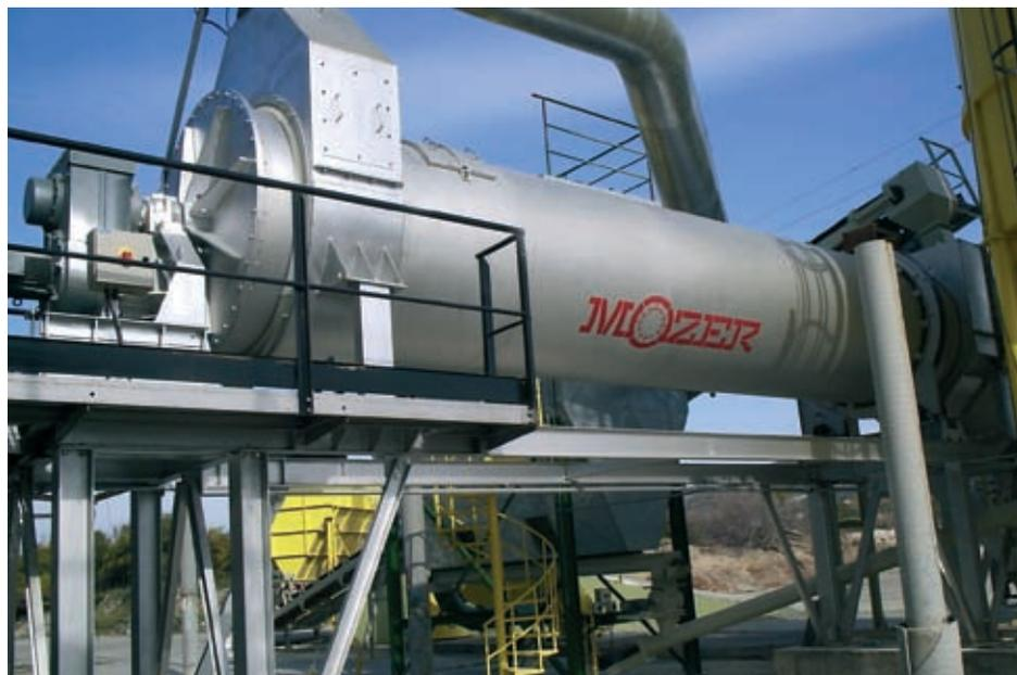
Drum dryer „System Mozer“ for drying limestone and diabase
