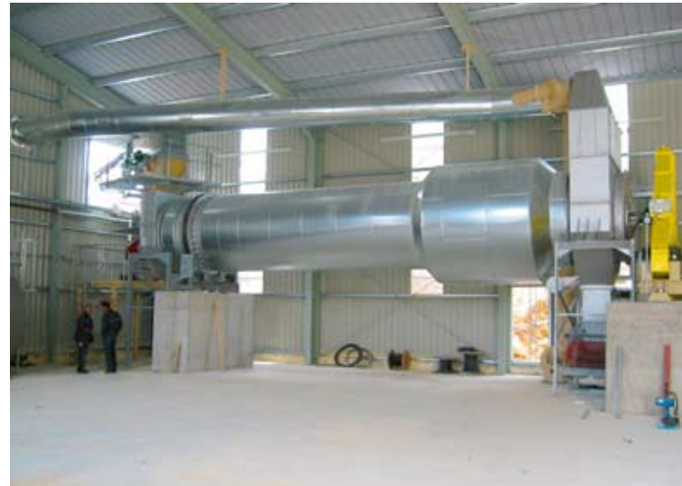
5 Trocken-Reinigungstrommel System MOZER®-TRH MOZER®-TRH system drying-cleaning drum
