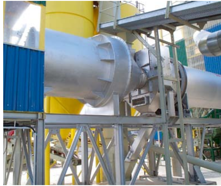
1 Brennkammer eines Trommeltrockners System MOZER® Firing chamber of MOZER® system drum dryer
